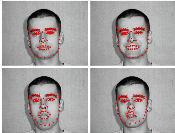
Figure 5: Real experiment results for deformation tracking. The key frames 1, 30, 138 and 190 shows different facial expressions of the subject. Red dots stand for the actual tracked positions.
