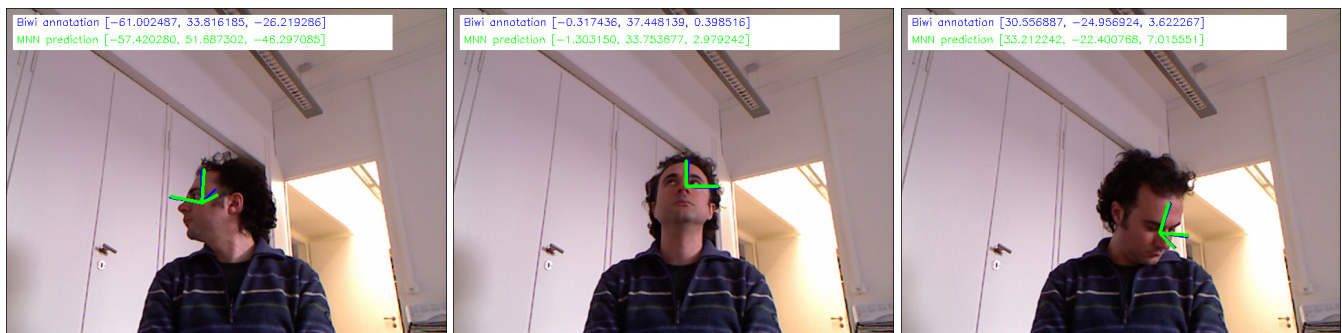
Fig. 4: Some processed frames from a Biwi sequence in laboratory conditions (see mnn.mp4). In blue and green we display respectively Biwi annotations and MNN predictions. Yaw, pitch and roll angles are also shown enclosed in brackets.
