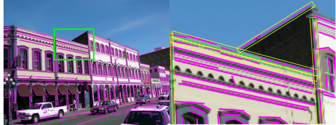
Fig. 1: Problem statement: Detected line segments are not usually collinear. Left: Line segments detected in an image using LSD (magenta lines). Right: Detected segments are not strictly aligned with straight scene lines (green lines). The smallest bounding box containing the segments of a scene line is plotted in yellow.
