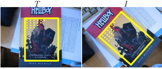
Fig. 1 Domains \mathcal{D} , \mathcal{V} , \mathcal{X} involved in an image alignment problem. \mathcal{D} depends on the domain in which the warping function is defined. Typical domains for this example would be \mathbb{R}^2 or \mathbb{P}^2 . (left) We overlay the target region \mathcal{V} (yellow square) onto the template T . The support set \mathcal{X} for the target region \mathcal{V} is given by the set of yellow dots. (right) We transform \mathcal{V} and \mathcal{X} into \mathcal{V}' and \mathcal{X}' by means of \mathbf{f} .
