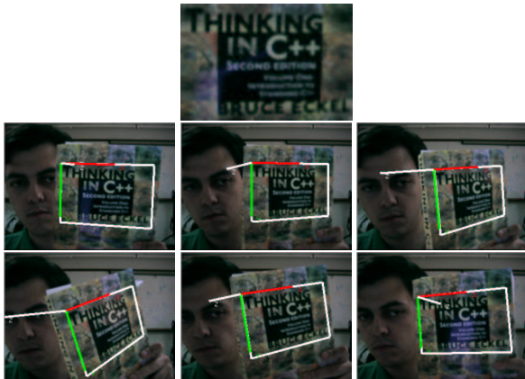
Figure 3. In the first row: template image. Second and third rows, frames 35, 84, 115, 170, 200 and 250 of 350. The white quadrangle is the position in 2D estimated from the projective SSD tracker. The 3D pose estimation: Z axis in white (out of plane), Y axis in blue and X axis in green.
