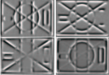
Fig. 2. Jacobian matrix for a translation (x, y) , rotation (\theta) and scale (s) motion model. In reading direction each image represents respectively I_x, I_y, I_\theta, I_s .
