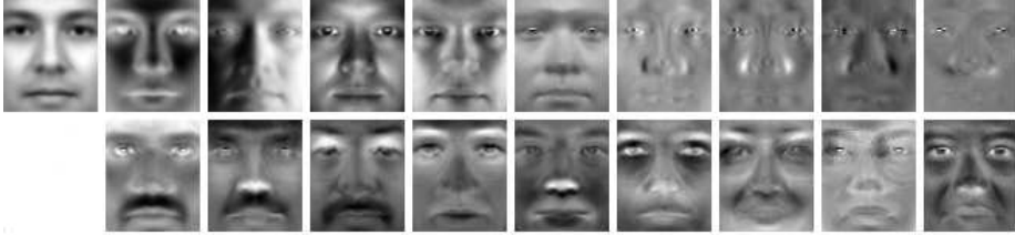
Fig. 3. Mean of illumination and identity training images (first image in first row). Illumination subspace basis vectors (remaining images in first row). Most significant components of the identity subspace basis (second row).
